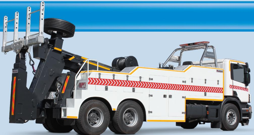
**Main Boom made from high tensile steel that is raised and lowered by double acting hydraulic cylinders**
